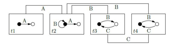
A synchronization scenario with 4 tasks synchronizing on 3 gates
