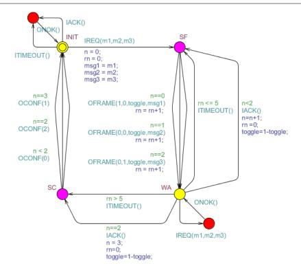
Fig. 6 Reference implementation of the BRP sender. The input symbols start with I, the output symbols start with O. In addition to symbols, the transitions contain value checks (or guards, ==, <, >) and assignments (=).
