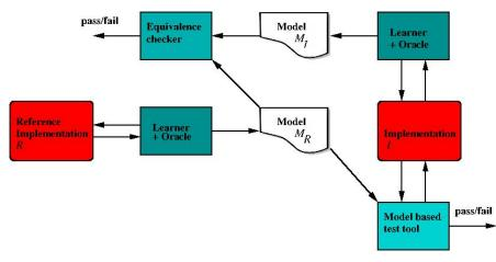
Fig. 4 Basic approaches of using automata learning to establish conformance of implementations. The learners interact with the implementations in order to construct models, which are then subsequently used for model-based testing or equivalence checking.
